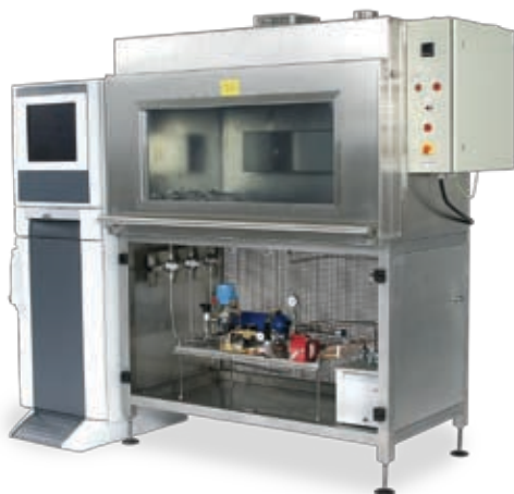
Burst Test Stand - Hydro-static testing of car radiator hoses
